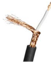
Unbalanced Cables have only one conductor per channel and a ground and therefore are highly susceptible to picking up noise.
